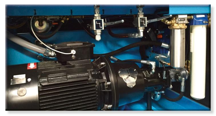
The final engineered solution for AMC Jets system consists of a portable data logger, four flow meters with on-board temperature, four pressure transducers, a particle counter and all relevant connectors and cables.
