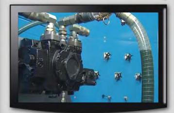
Run oil through the pump and display real-time hydraulic values (Flow, pressure, temperature, speed plus custom analog measurements)
