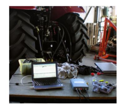
Those who needed a lower-cost, low-tech tool for measuring flow pressure and temperature in smaller (sub 60 horse power) machinery
