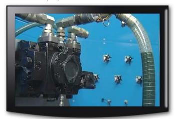
Run oil through the pump and display real-time hydraulic values (Flow, pressure, temperature, speed plus custom analogue measurements)
