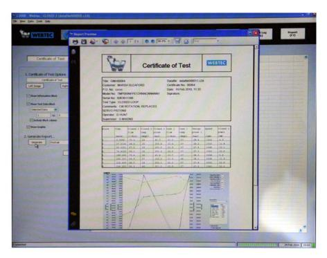
Because the test certificates produced by the C2000 cannot be manipulated, but are a true representation of the test carried out, GM Hydraulics and its customers have total assurance that any pump which is tested is in perfect working order when it leaves GM's premises. Not only does this mean no disputes concerning the test itself, but should a fault develop at a later date, the stored data can be recalled and the constancy of values checked, which greatly assists in the diagnostic process.
