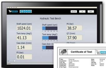
Using your own test procedure you can display real time values and record test results on a keypress
