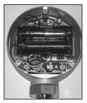
When in continuous operation (without light), the service life of the batteries is 1,500 hours.
