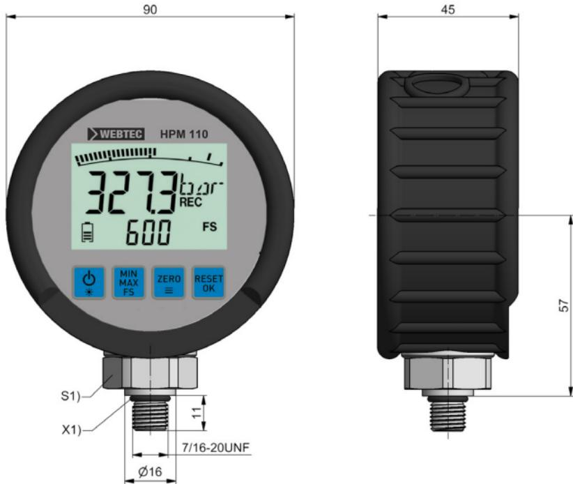
Fig. 3: Dimensional drawing SR-HPM-110-UN
