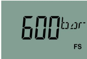
Display of the measuring range (FS) in bar.
