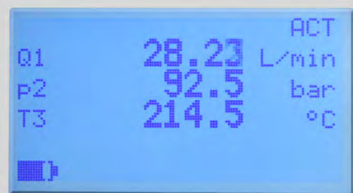
HPM540 displaying flow, pressure and temperature
