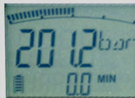
HPM110 showing actual pressure as numeric value and on bar graph
