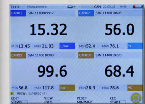
HPM6000 showing four large numeric values (press down to show additional values)
