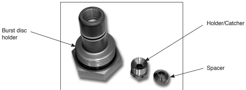
Using new burst discs (one either side of the burst disc spacer - see step 3) insert one into the holder/catcher, followed by the burst disc spacer and then the second burst disc. Screw the burst disc holder/catcher back into the top of the holder body and tighten to a torque of 55 Nm (40 lb/ft).
