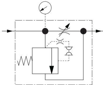
**Note:** There is only a highly restrictive path through the valve for reverse flow - the burst discs will blow via the pilot exhaust line but the bypass valve will not operate.
