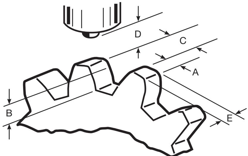
The above configuration is usually not available in a stock gear, but it is not necessary to have the maximum output into the conditioning. Conventional stock gears can be used if the tooth width A is equal to or greater than 2.3mm and C is 3.5mm. For ease of alignment, it is recommended that the gear thickness should be at least 5mm.
